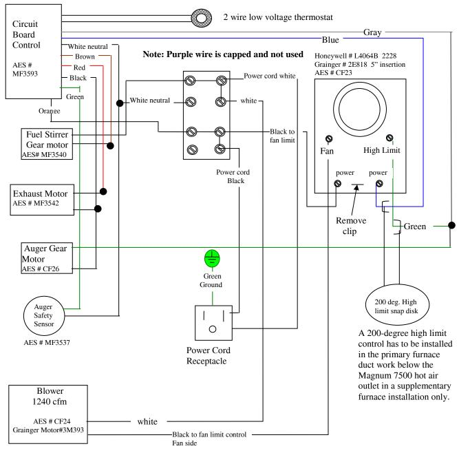
**IMPORTANT:** Incorrectly installed fan limit controls can cause electrical shock, shorting out of the circuit and damage to the unit. **The Brass jumper wire must be removed on the fan limit control**. Refer to the installation, setting and operation instructions provided with the fan limit control.
