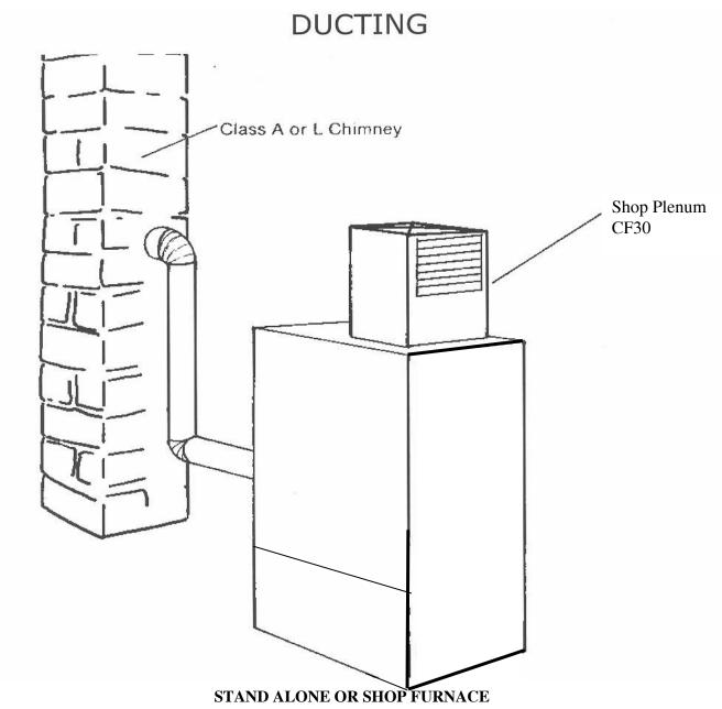
The Magnum 7500 Corn/Wood Pellet Furnace may be installed as a stand-alone system as long as the unit is in a non-confined area. An unconfined space would be an area with 8' ceiling height minimum and 650 square feet minimum open floor space. Fresh Air for combustion would have to be connected directly to the furnace and adequate infiltration for dilution and distribution of supply and return air would have to be provided.
