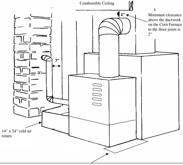
Floor protection must be provided because of possible spillage of ashes and burning fuel. There must be non-combustible materials placed 6" in front of and 6" to the side of the fuel loading and ash removal doors. If the unit is setting on a cement floor no protection is needed. Consult your local dealer for possible sources for non-combustible materials acceptable to be used.
