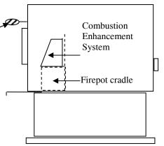
The combustion enhancement system sits on top of the Firepot. When starting the fire use the scraper tool and remove the CES to expose the firepot. Make sure that there is not fuel or ashes on top of the firepot flange when re-installing the combustion enhancement system.
