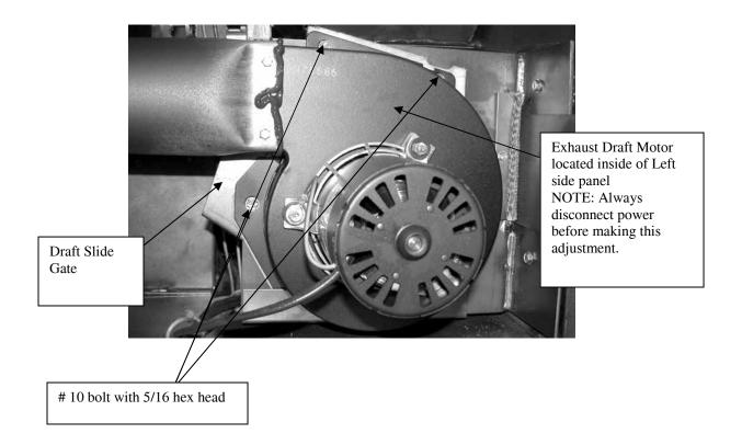
The normal operation of the Magnum 7500 would be with the Draft Slide Gate open fully as shown. When the gate is in the fully open position, the plate will be against the mounting plate as shown. If the unit needs a draft correction adjustment, the bolts are loosened and the slide gate is rotated a few degrees at a time until the proper operation of the unit is achieved.
