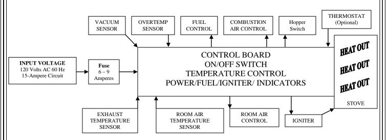
The basic block diagram shows the input and output components to the control board. The failure of any of these items to work properly will cause a malfunction in the system. Further information on each function is provided in the tables below.
