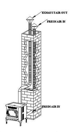
FIGURE 8: CHIMNEY FLUE AND FRESH AIR VENTING
