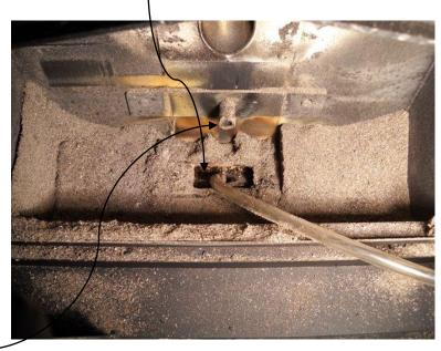
Clean the area around the igniter tube and carefully clean the end of the igniter of any buildup.
