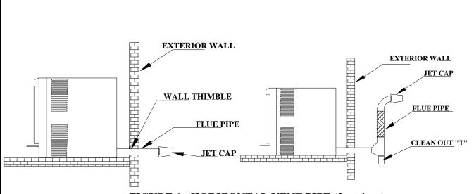
FIGURE 1: HORIZONTAL VENT PIPE (2 options)
