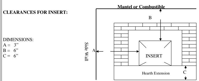
FIGURE 7: INSERT MINIMUM CLEARANCES
