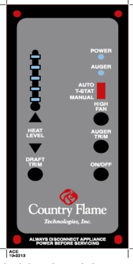
NOTE: Priming the auger is required when the unit is new or when the hopper has completely run out of fuel. This can be done approximately 1 minute after pushing the on/off start button. Press and hold the "auger" button until fuel begins to drop into the firepot. When fuel begins to drop regularly, release auger button, the auger is primed.
