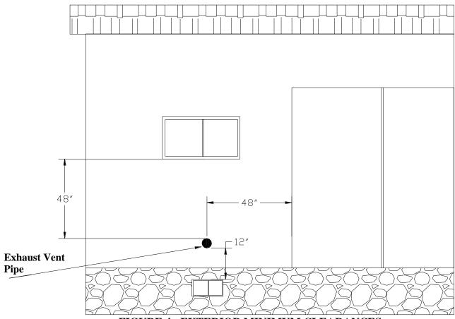
FIGURE 4: EXTERIOR MINIMUM CLEARANCES
