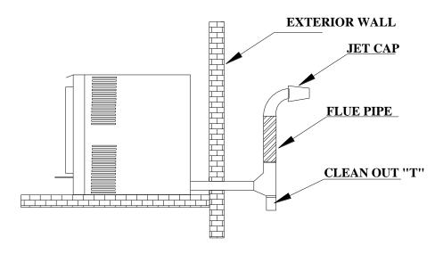
FIGURE 3: RECOMMENDED EXTERIOR WALL INSTALLATION
