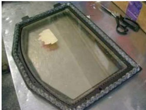
4. Secure glass in place with clips and screws. Use the drawing below to tighten the screws in the sequence marked. Tighten screws to 10Kg/cm.
