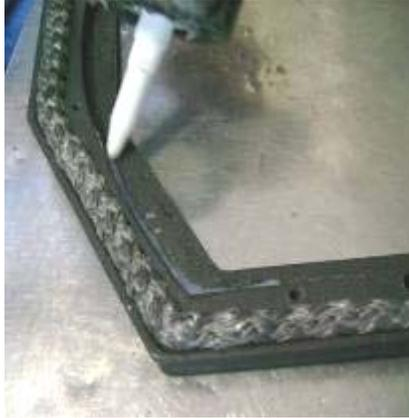
2. Press R-133 rope gasket into the silicone using a slight back and forth motion to make sure the silicone is pressed into the rope. Trim and tuck ends as with outer gasket.
