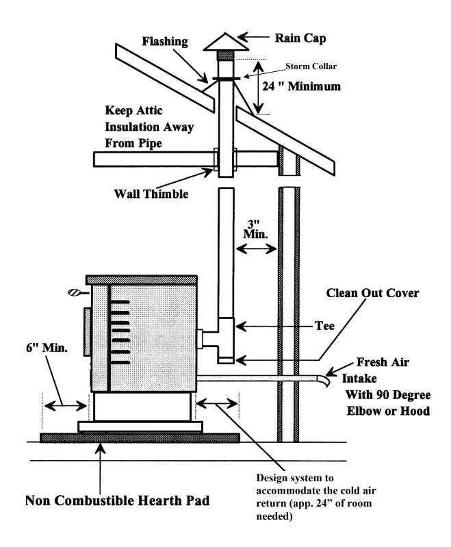
INSIDE VERTICAL PIPE WITH ROOF TERMINATION
