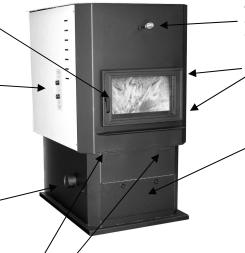
Ash clean outs Pull out to empty ashes out of firebox area and back heat exchanger area. Make sure to push all the way in when done.
