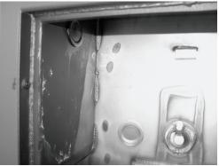
plates, be sure to re-install them. If they keep falling out replace them with new ones. Do not operate the unit without them installed. If you are having trouble contact your local service technician for help.
