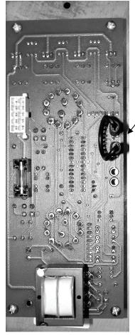
Two (2) <sup>1</sup>/4" male spade connectors, one for each wire from wall thermostat
