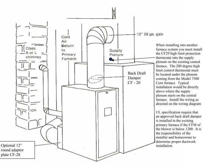
Add-On Furnace (Supplementary Heat installation)
