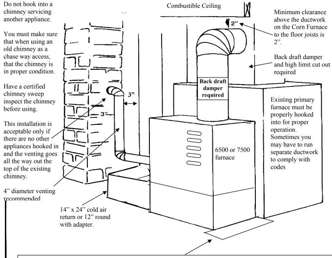
Floor protection must be provided because of possible spillage of ashes and burning fuel. There must be noncombustible materials placed 6" in front of and 6" to the side of the fuel loading and ash removal doors. If the unit is setting on a cement floor no protection is needed. Consult your local dealer for possible sources for non-combustible materials acceptable to be used.
