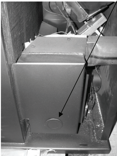
Auto Reset 110 deg Normally open Cool Down
