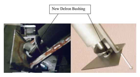
**What to look for:** There has been a new delron bushing with a longer flange that extends toward the auger motor installed between the auger and auger plate. This is to help alleviate the play between the auger and auger plate so that the bushing does not fall out of the plate.
