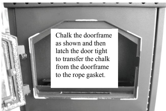
Chalk the doorframe as shown and then latch the door tight to transfer the chalk from the doorframe to the rope gasket.
