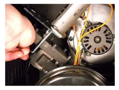
• Slide the motor shaft into the auger shaft
