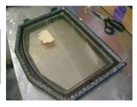
4. Secure glass in place with clips and screws. Use the drawing below to tighten the screws in the sequence marked. Tighten screws to 10Kg/cm.
