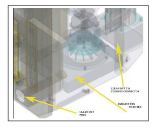
The chimney adapter can be removed by taking out the 4 hold down bolts as shown. Cleaning this area of the insert is part of the recommended yearly maintenance. The system can be cleaned from atop the chimney. By using the reverse suction of a powerful leaf blower, all ash from the exhaust chambers can be removed easily. The unit can be pulled out of the fire place to remove the adapter, and then ash-vac the exhaust box out.
