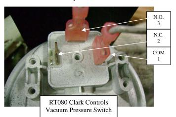
Attach one grey wire to 'Com 1' and one grey wire to 'NO 3'. Attached hose to bottom connection 'H'. ♦ The RT080 World Magnetics Vacuum Pressure Switch is installed vertically to the base of the stove, with 2 screws (#8 x 1/2 tek, ZP 1/4" hex head).
